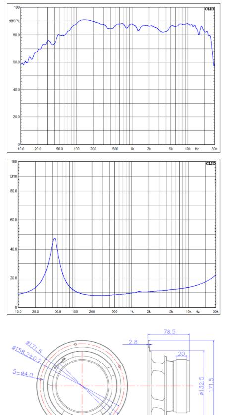
FS: 44.1601 Hz VAS: 24.7335 L RE: 6.8000 Ω L1kHz: 0.2771 mH L10kHz: 0.1229 mH X Max 8mm 1 way Pwr: 45watts Nom
