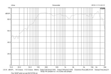
VAS 1.2475 L RE 3.3000 Ohm QMS 2.723 QES 0.7084 QTS 0.5621 2.2925 Txm Bxl SPL 87.5192 SD 0.0028 m2 CMS 1.1175 mm/N MMS 1.4224 g RMS 0.4143 WM RAT 251048 WA RMT 2.0070 WM MMD 1.3373 g 0.34% h0 L1kHz0.0599 mH PWR 7 watts (Nom) X MAX (Mech) +/- 3.5mm
