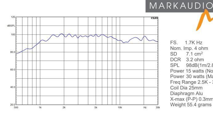
FS. 1.7K Hz Nom. Imp. 4 ohm 7.1 cm<sup>2</sup> SD DCR 3.2 ohm SPL 98dB(1m/2.83W) Power 15 watts (Nom) Power 30 watts (Max) Freq Range 2.5K - 30K Hz Coil Dia 25mm Diaphragm Alu X-max (P-P) 0.3mm Weight 55.4 grams
